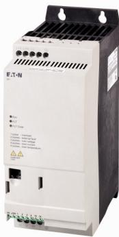
**Variable speed starter, Rated operational voltage 400 V AC, 3-phase, Ie 6.6 A, 3 kW, 3 HP**
